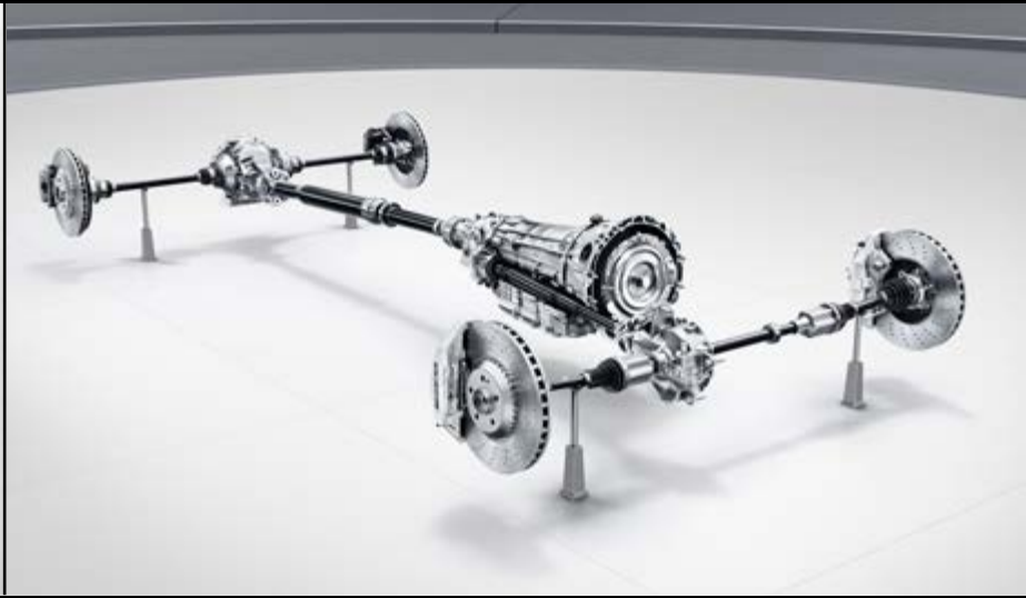
Propulsione integrale AMG Performance 4MATIC+
